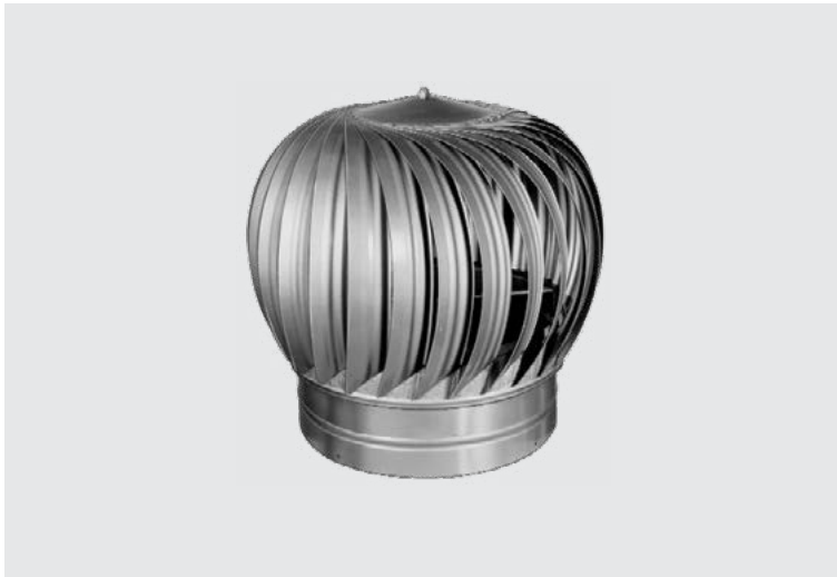
TURBINE VENT Model RR turbine vents provide consistent warm air exhaust for smaller spaces. The spinning turbine head draws hot air out of the building. Exhausted air and ambient wind spin the turbine head.
